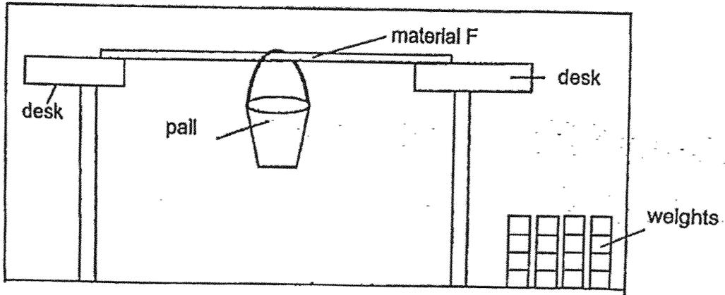
He placed the weights into the pail one at the time until the material F broke. He repeated the experiment with material G and H and recorded his results in the table below.
